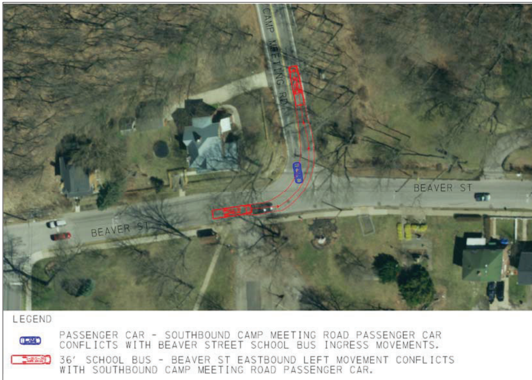
Turning simulation showing the school bus turning left into Camp Meeting Road
