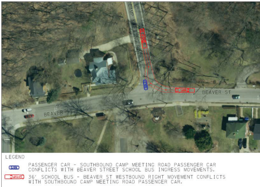
Turning simulation showing the school bus turning right into Camp Meeting Road
