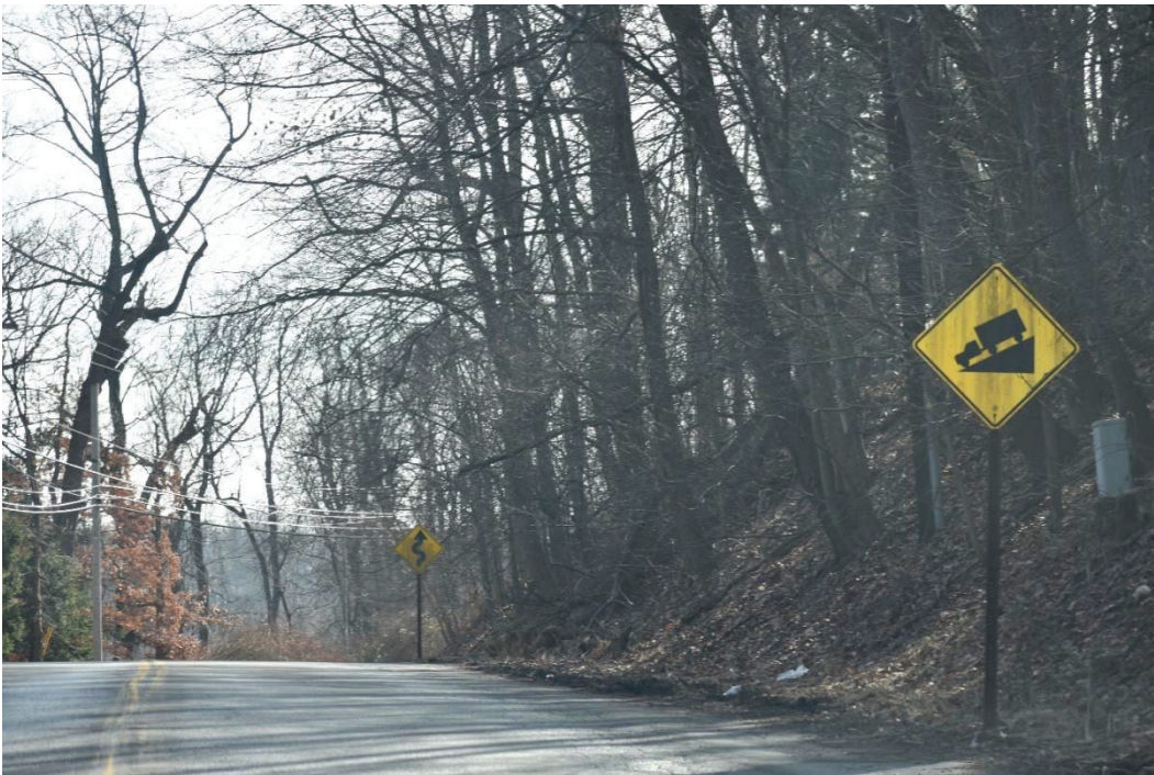
Hill (W7-1) and Winding Road (W-15) signs on southbound Camp Meeting Road approaching the school area
